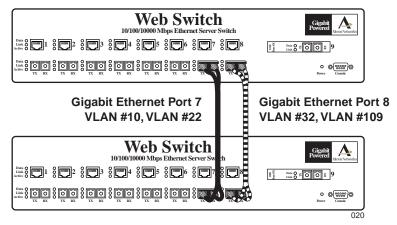
Figure 2-2 Example 2: Parallel Links with VLANs
